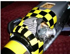
As previously stated I have gone for a large motor, this being the Zenoah 45cc petrol witch needed to be shoe horned into the cowl, alas the silencer is large and ugly but I have sought of got used to it and I have simply not been able to find a better solution at this time.
