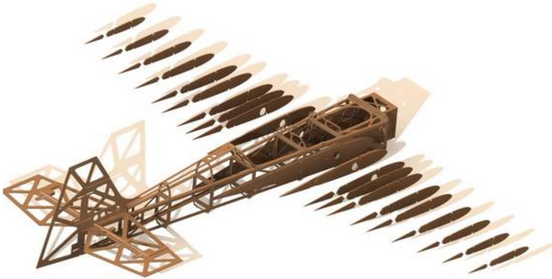
The model will have a wingspan of 1800mm (70") a total length of 1750mm and Mike is hoping for a weight of around 9lbs all up, with a target wing loading of 18oz per square foot, the model is going to be all electric and will be powered by Tornado Thumper 2.5KW motor swinging a 20" prop, and it will all be fed through a 120A speed controller and a 10 cell 5350mAh lithium polymer battery which he hopes will give him a flying time of around 8 – 10 minutes.
